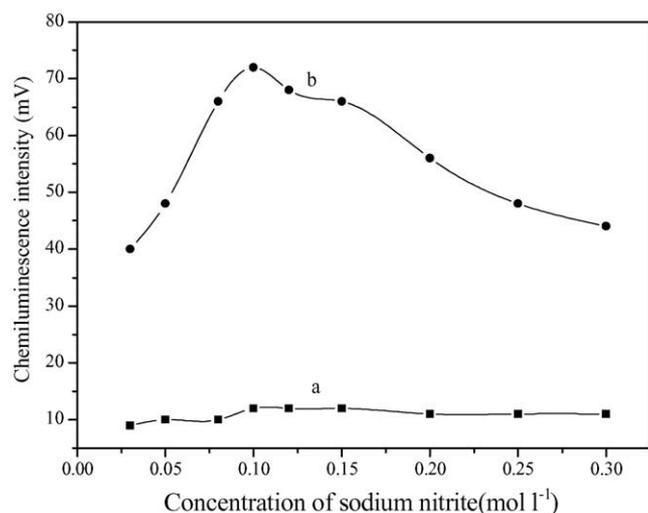
Fig. 6. Effect of sodium nitrite concentration on the chemiluminescence intensity in  $0.25 \text{ mol l}^{-1}$  hydrogen peroxide– $0.20 \text{ mol l}^{-1}$  sulfuric acid in the absence (a) and the presence (b) of  $2.0 \times 10^{-6} \text{ mol l}^{-1}$  tryptophan.
