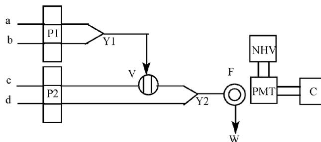
Fig. 1. Schematic diagram of the flow-injection chemiluminescence manifold used for the determination of tryptophan: P1 and P2, peristaltic pump; Y1 and Y2, three-way pipe; V, six-way valve; F, flow cell; W, waste; NHV, negative high voltage; PMT, photomultiplier tube; C, computer; a, sample stream; b, sodium nitrite stream; c, sulfuric acid carrier stream; d, hydrogen peroxide stream.
