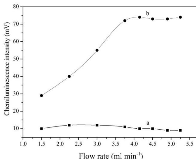
Fig. 7. Effect of flow rate on the chemiluminescence intensity in  $0.10 \text{ mol l}^{-1}$  sodium nitrite– $0.25 \text{ mol l}^{-1}$  hydrogen peroxide– $0.20 \text{ mol l}^{-1}$  sulfuric acid in the absence (a) and the presence (b) of  $2.0 \times 10^{-6} \text{ mol l}^{-1}$  tryptophan.
