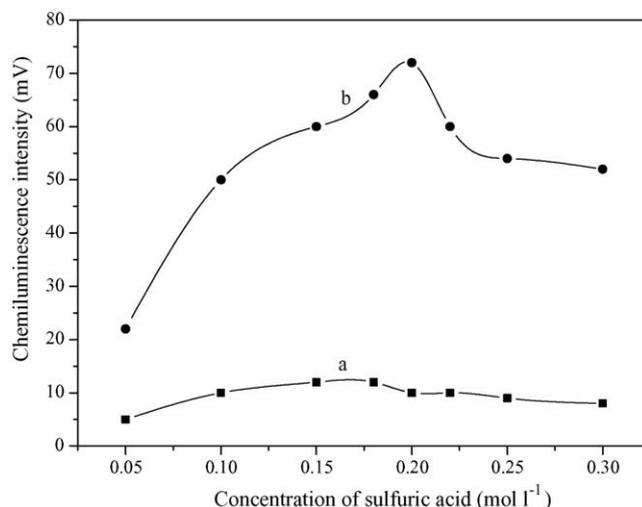
Fig. 4. Effect of sulfuric acid concentration on the chemiluminescence intensity in  $0.10 \text{ mol l}^{-1}$  sodium nitrite– $0.25 \text{ mol l}^{-1}$  hydrogen peroxide in the absence (a) and the presence (b) of  $2.0 \times 10^{-6} \text{ mol l}^{-1}$  tryptophan.
