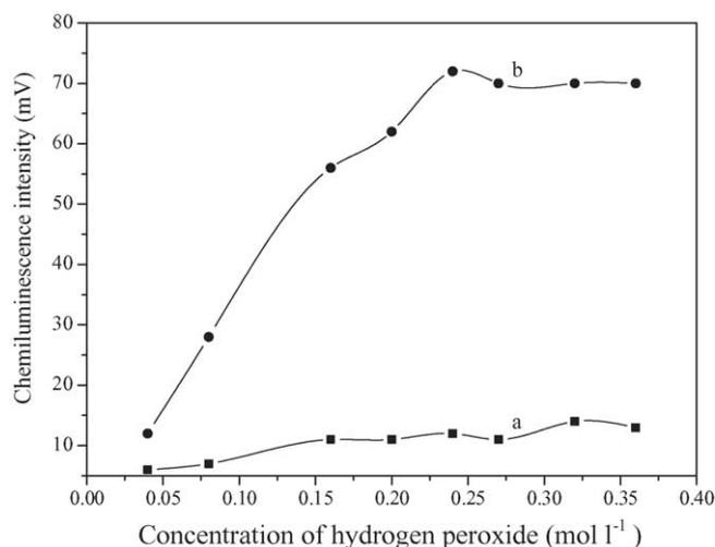
Fig. 5. Effect of hydrogen peroxide concentration on the chemiluminescence intensity in  $0.10 \text{ mol l}^{-1}$  sodium nitrite– $0.20 \text{ mol l}^{-1}$  sulfuric acid solution in the absence (a) and the presence (b) of  $2.0 \times 10^{-6} \text{ mol l}^{-1}$  tryptophan.
