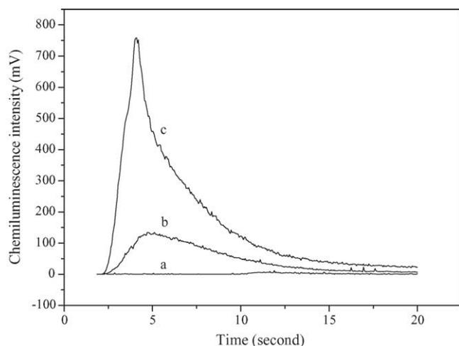
Fig. 2. Chemiluminescence dynamic response curves of chemiluminescence reaction of  $0.25 \text{ mol l}^{-1}$  hydrogen peroxide– $0.20 \text{ mol l}^{-1}$  sulfuric acid with (a)  $2.0 \times 10^{-6} \text{ mol l}^{-1}$  tryptophan, (b)  $0.10 \text{ mol l}^{-1}$  sodium nitrite and (c)  $0.10 \text{ mol l}^{-1}$  sodium nitrite and  $2.0 \times 10^{-6} \text{ mol l}^{-1}$  tryptophan in batch mode.
